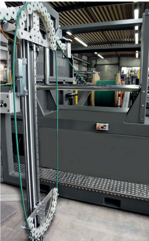
Fig. 2 ACUMATIC, material accumulator / dancer for controlling and synchronization of the drive of the drum. Necessary for tension sensitive winding goods
