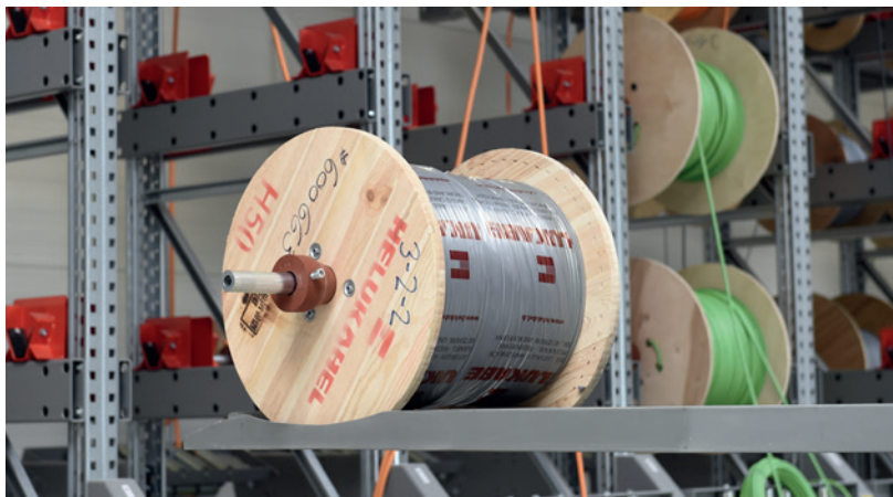
Fig. 2 TROMPLAT 1000 example of storing the drum into a Kabelmat LAGROL rack
