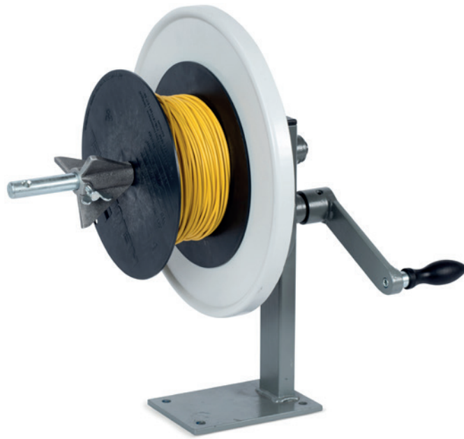
Fig. 1 TISCHROL Complete device TISCHROL 1:3 with spool winding axle
