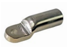
HELU-S-PK-AL-FG-VZN Aluminum, tinned, FG, extruded, straight ring design Part no. 909853
